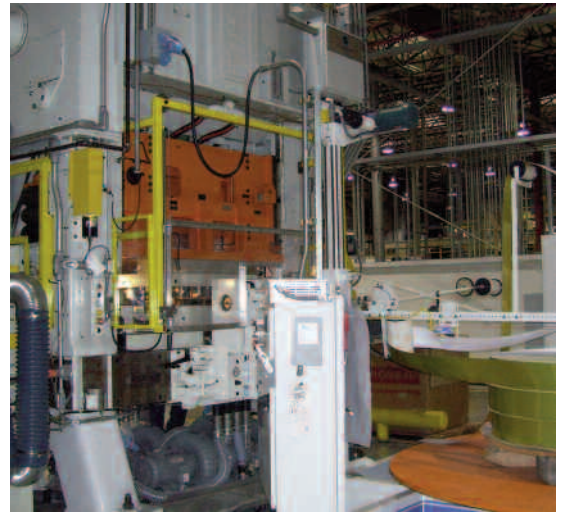
Power to the uncoiler in front of this Stolle Cupping System can be disconnected easily for die changing or maintenance, using the Meltric Decontactor visible above the die on the left side of the machine.
