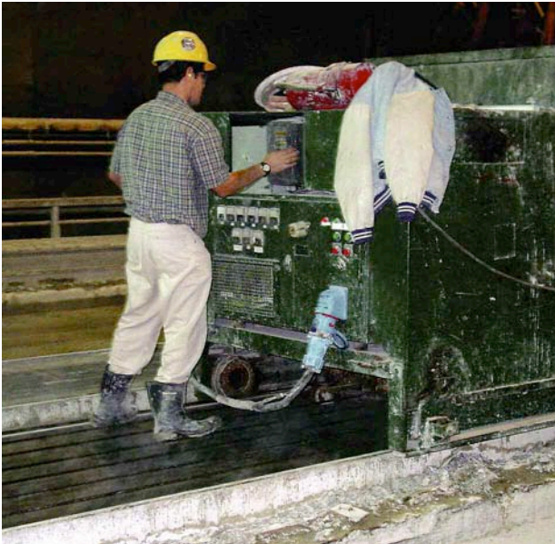
DS60 equipped power cables provide a safe and convenient means of routinely making and breaking power supply connections as required while this concrete floor panel forming machine moves along the production line.
