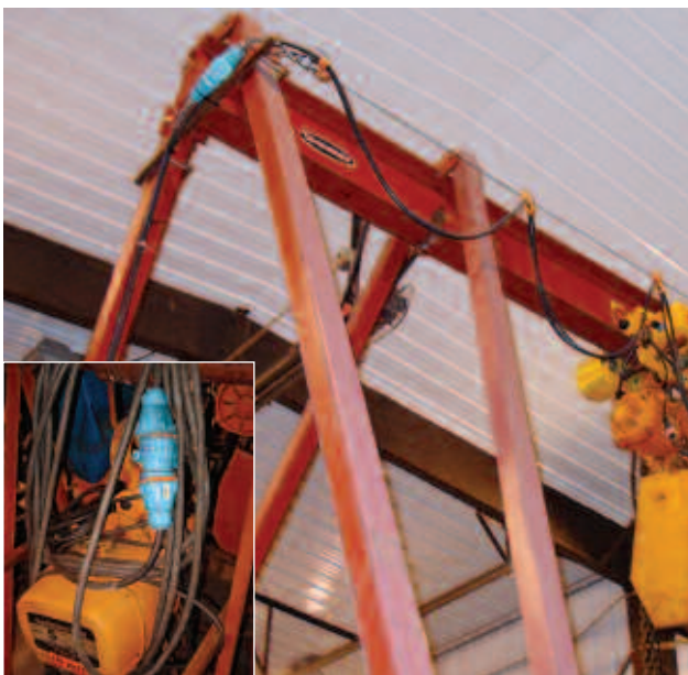
Decontactors used as in-line disconnects facilitate quick and safe servicing of hoist equipment.
