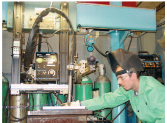
EWI Technician sets up a gas metal arc welding torch powered via a switch rated Deconnector plug and receptacle.
