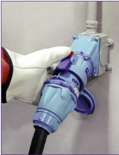
Pressing the pawl on the DECONTACTOR receptacle breaks the electrical connection. The de-energized plug can then be safely withdrawn.
