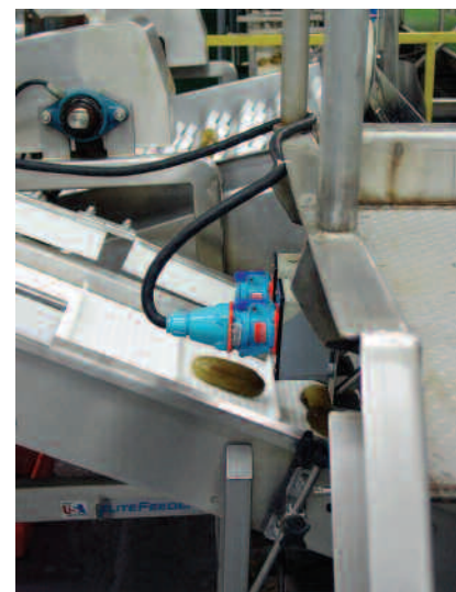
Decontactor plugs feature an OFF switch/pawl which can be used as an emergency disconnect switch for conveyors.
