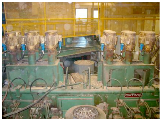
Closeup shows typical motors with Meltric Decontactors in place. Dead-front construction keeps workers safe, while plug-and-play simplicity speeds motor removal and reinstallation.
